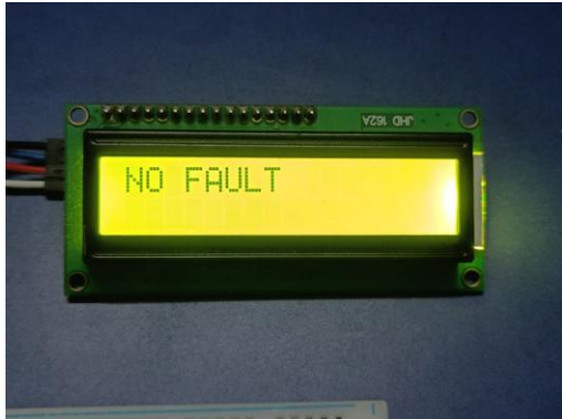
Fig 3: LCD Display Indicating Normal Operating Condition (No Fault Detected)
